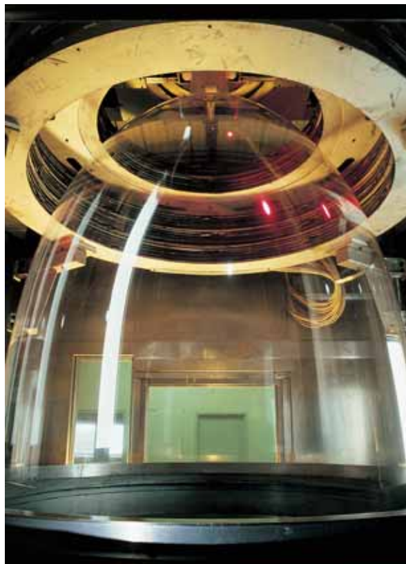
Innovia Films unique and proprietary "bubble process" produces high performance polymer for banknotes
