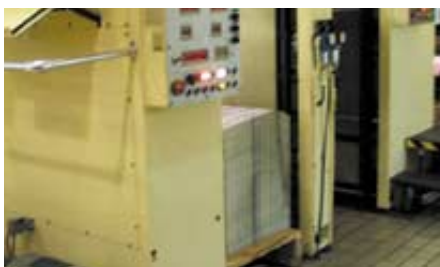
Printed sheets after the offset printing process waiting to be sent to the strong room to cure.
